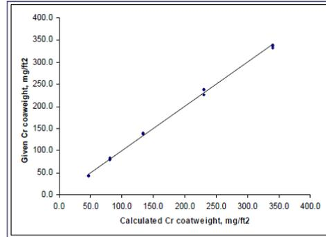
Figure 1: Calibration graph for Cr coatweight on aluminium
